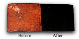
**Q 2** is a complex polymer coating containing a high molecular weight organic complex in a special non-corrosive acid base. It is designed to treat rusty iron-based metals to a protected, coated surface.
